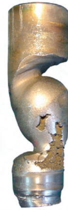
Fig. 6. Damage of valve due to flashing
