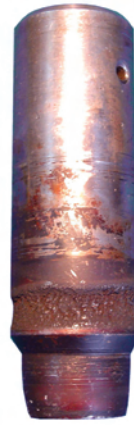
Fig. 5. Damage of valve due to cavitation
