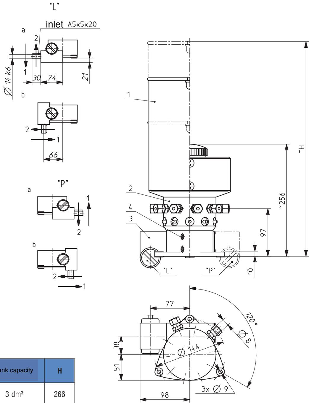
Fig. 6 Grease and oil lubrication pump with drive and additional reduction gear of MPS 10-C type
