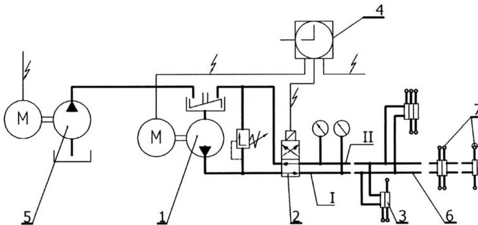
Fig. 1 Construction diagram of the two-way force feed oiling systems
