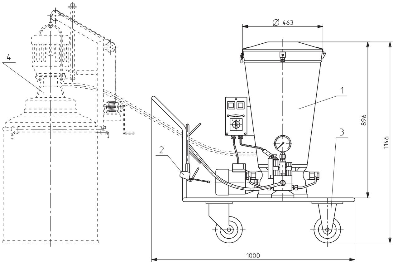
Fig. 2 Overall dimensions of the lubrication stand SA 1
