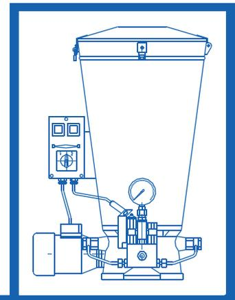
Central lubrication pump PD 12 & PA 12G
