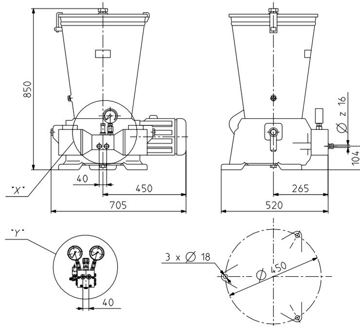
Fig. 3 Overall and linkage dimensions of the pump
