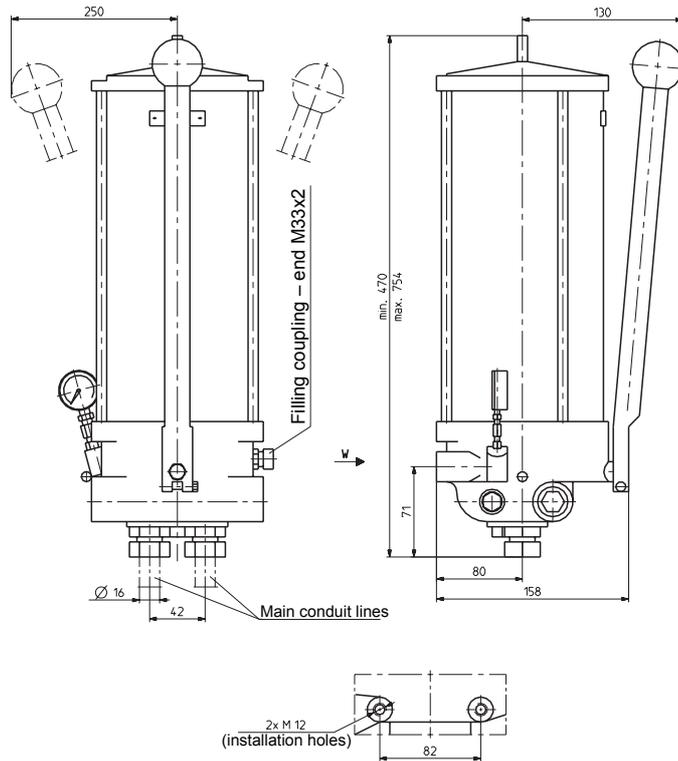
Fig. 1 Overall and linkage dimensions of the pump
