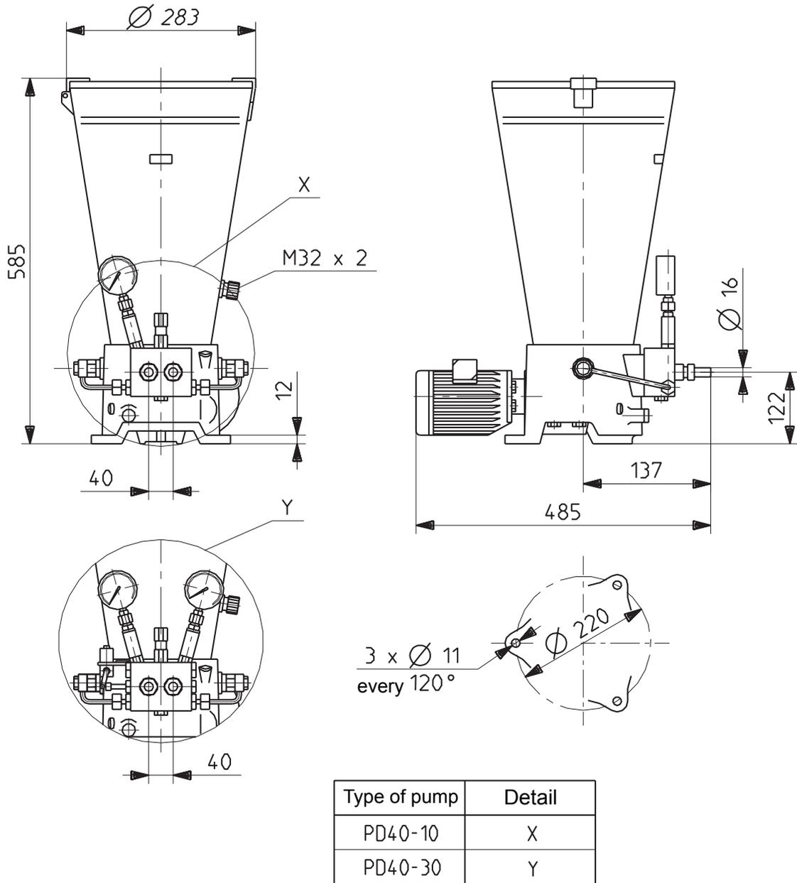
Fig. 3 Overall and linkage dimensions of the pump
