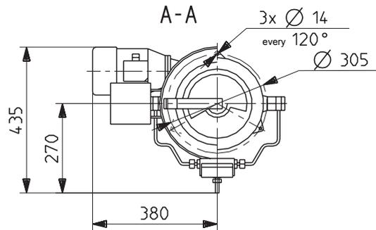
Fig. 2 Overall and linkage dimensions of the pump PA 12
