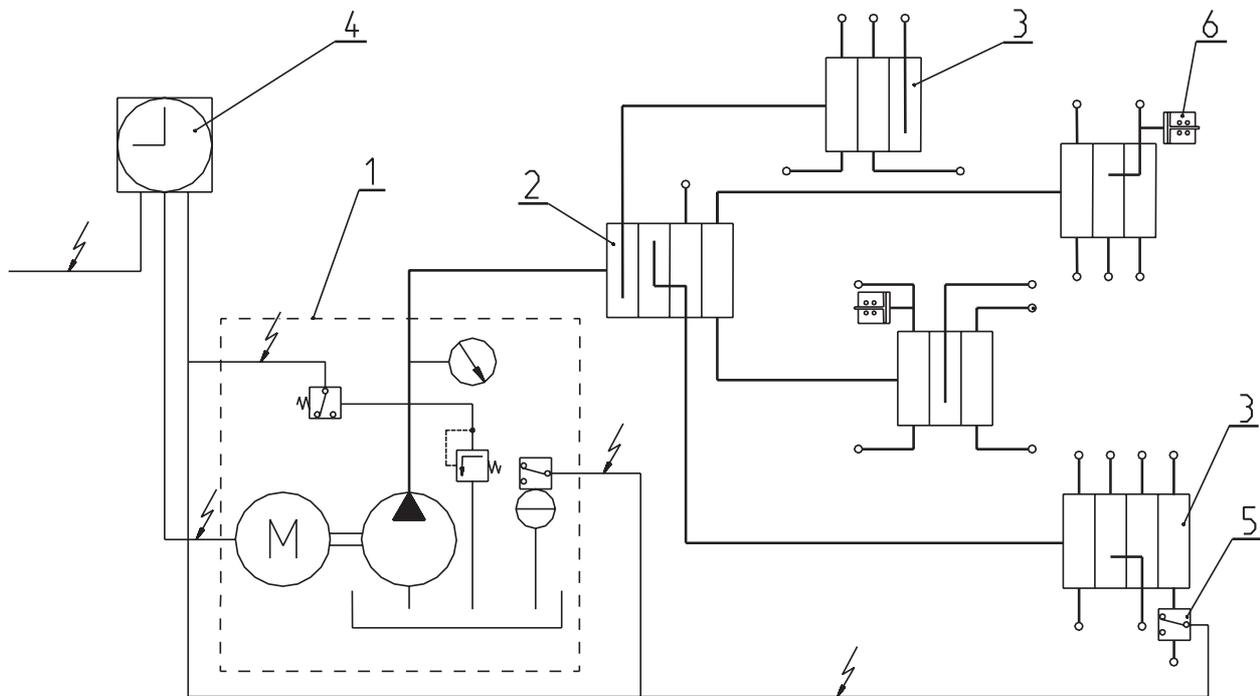
Fig. 3 Example scheme of a progressive force feed oiling systems
