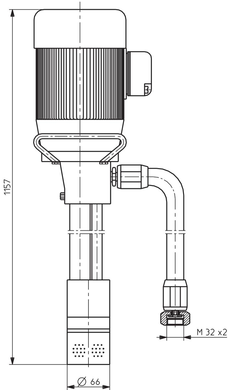
Fig. 1 Dimensions of the pump
