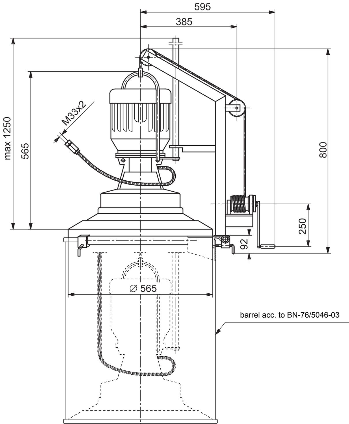
Fig. 1 Overall dimensions of the pump PZ 31
