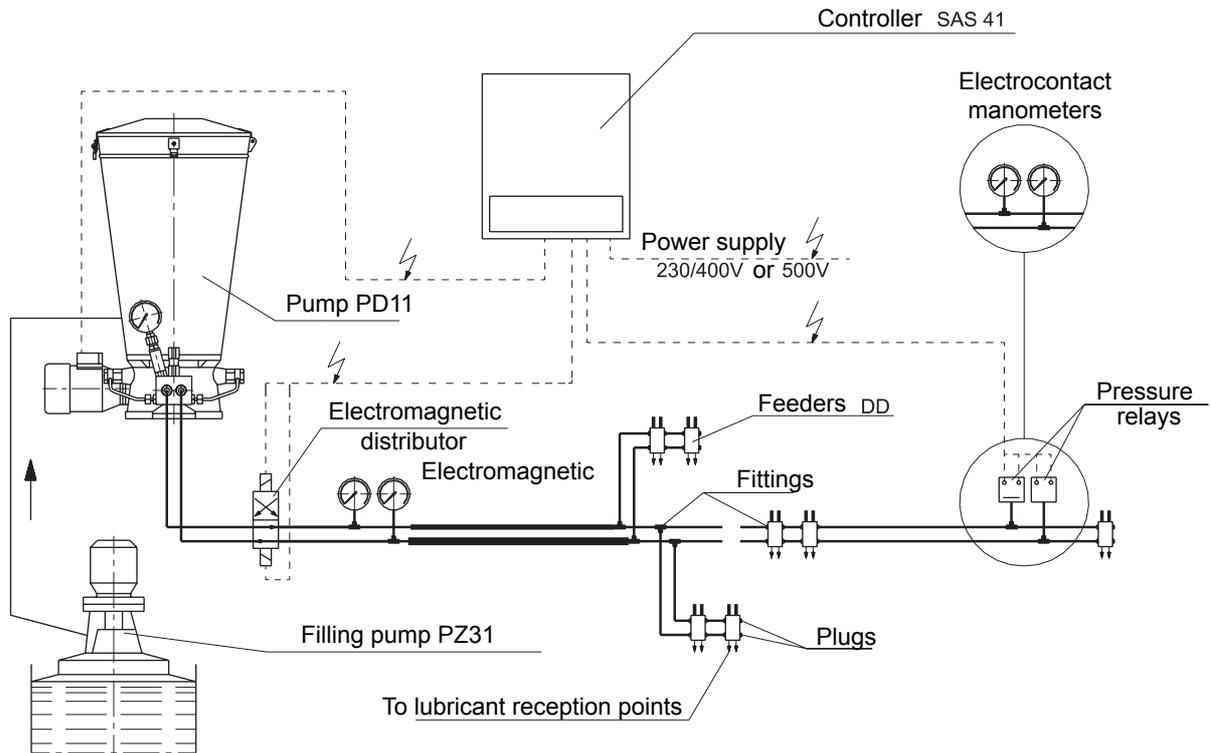
Fig. 2 Construction diagram of the central lubrication system with a PD 11 pump
