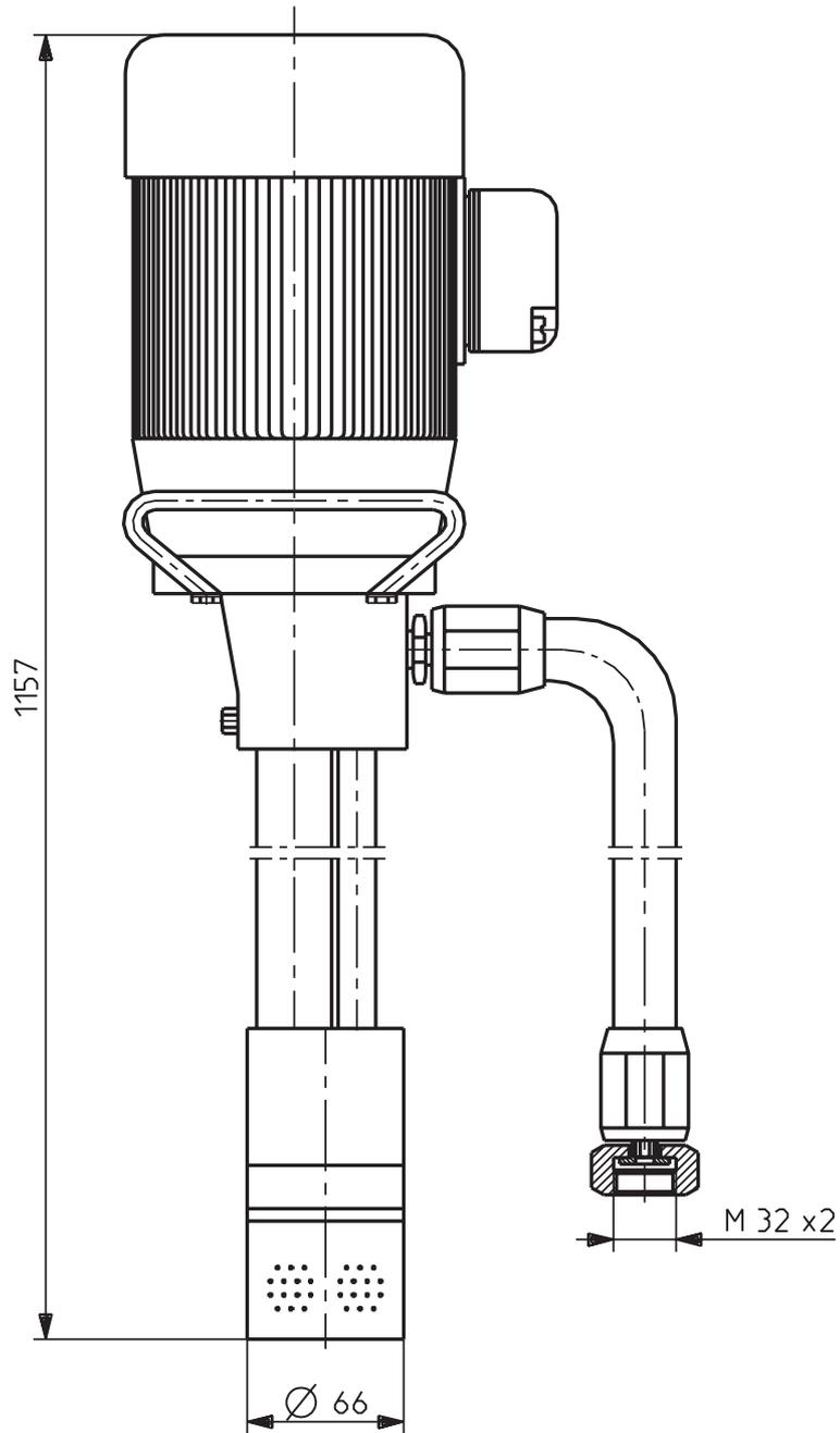
Fig. 1 Dimensions of the pump
