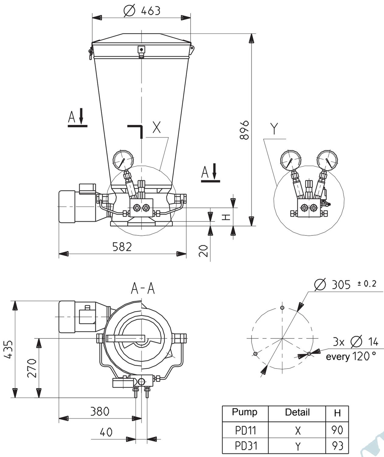
Fig. 1 Central lubrication pump of PD 1 & PD 11 type
