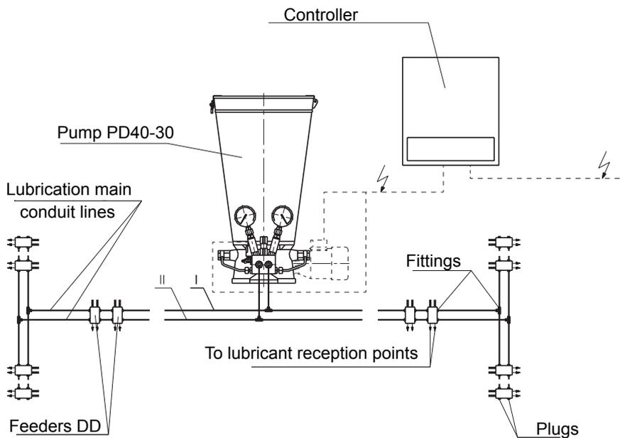
Fig. 2 Construction diagram of the central lubrication system with a PD 40-30 pump
