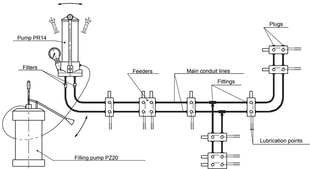
Fig. 2 Example scheme of an oiling system
