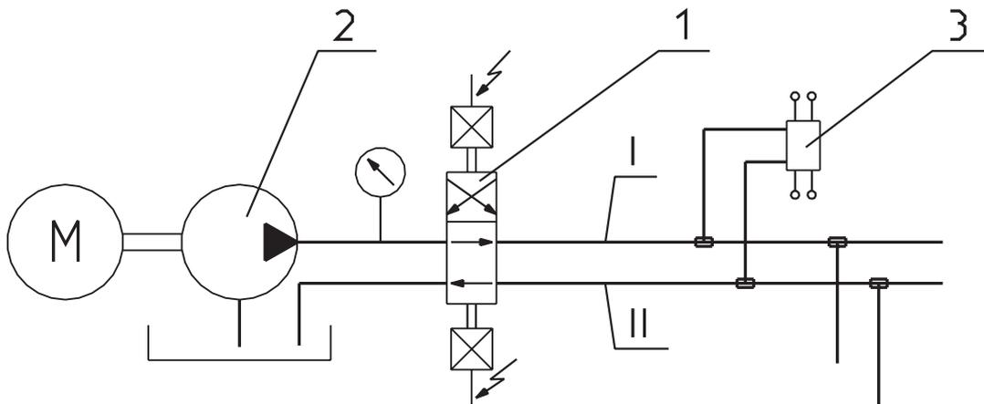
Fig. 1 Scheme of a lubrication system with the electromagnetic distributor
