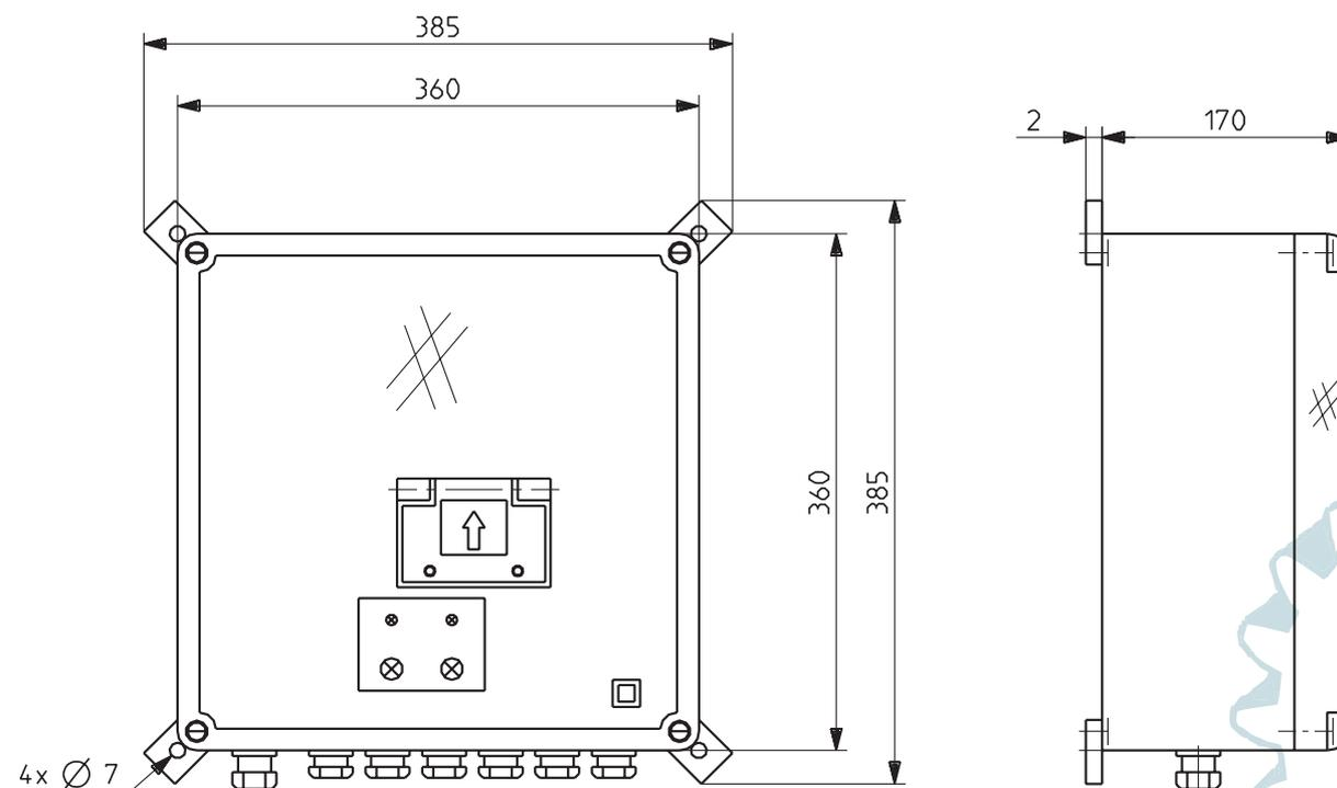
Fig. 5 Overall and linkage dimensions of SAS41; 42
