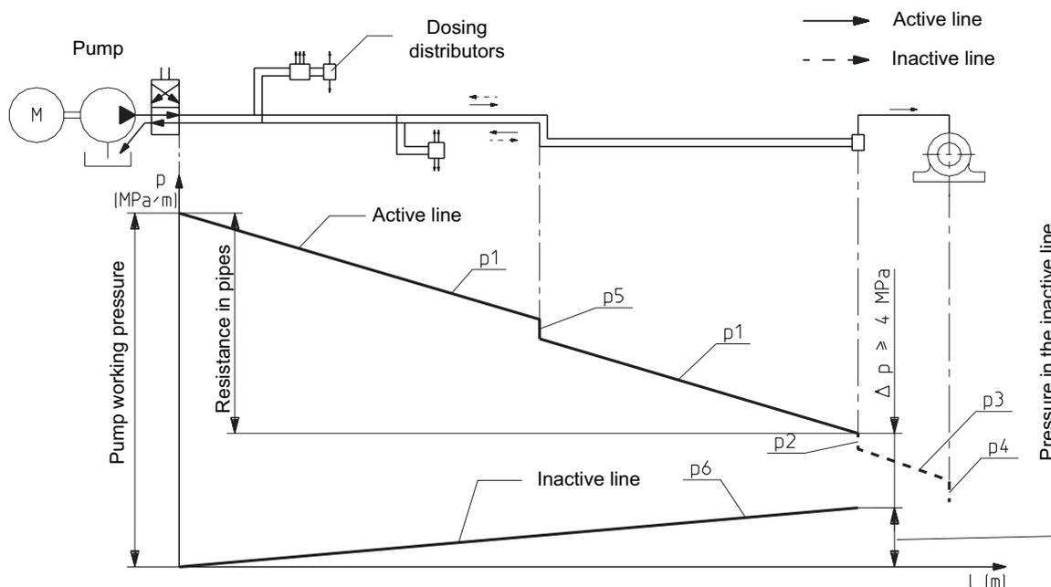
Fig. 3 Diagram of pressure drops in the lines of the central lubrication system.
