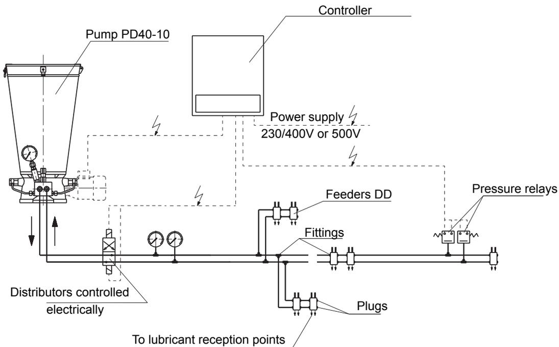
Fig. 1 Construction diagram of the central lubrication system with a PD 40-10 pump
