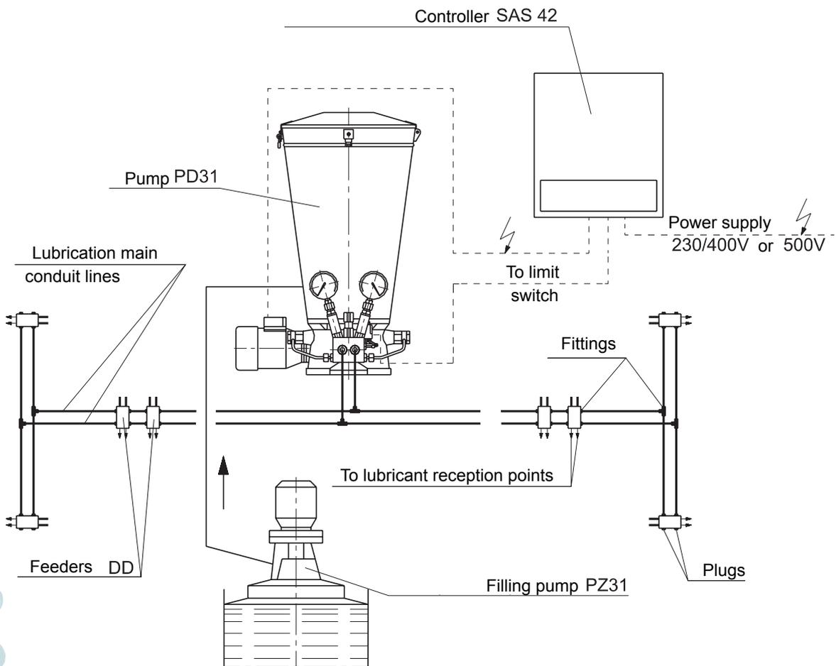
Fig. 3 Construction diagram of the central lubrication system with a PD 31 pump
