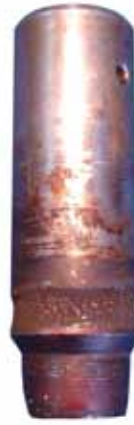
Fig. 5. Damage of valve due to cavitation
