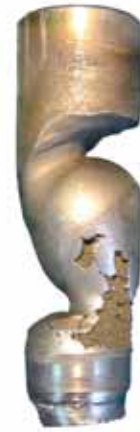
Fig. 6. Damage of valve due to flashing
